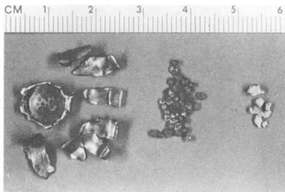
FIG. 11—Case 2: photograph of Glaser Slug fragments demonstrating extensively disrupted shot cup, dozens of shot, and fragments of the plug. Note that base of cup has retained a nearly circular configuration.
