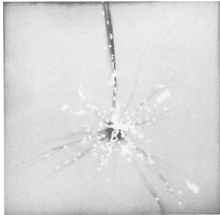
FIG. 20— Gelatin Block 4: Cross-sectional radiograph revealing large radial permanent cavity, dispersion of shot, and markedly fragmented shot cup.
