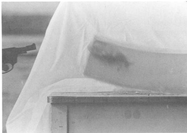
FIG. 21— Gelatin Block 5: Photograph depicting Charter Arms revolver recoil, movement of gelatin block, and permanent cavity within the block.
